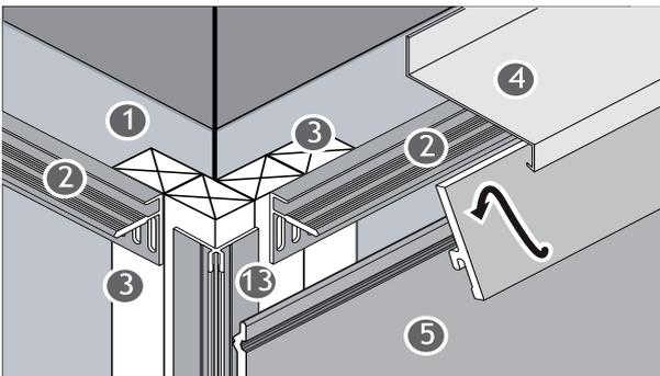
Fix vented starter/closer trim. Refer to Diagrams 7 & 8. Cut your cladding plank using the formula given.
