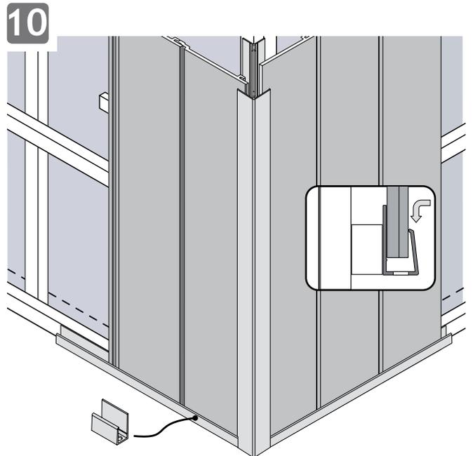
Slot the first row of cladding planks into the vented starter trim. (or starter trim) Allow expansion gaps at all edges and junctions. See Diagrams 11, 12, 13 & 14. Do not drive the screw or nail through the surface of the cladding as this will prevent the plank from moving if it expands.
